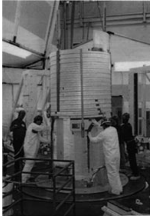
Figure 6. ITER CS model coil after heat treatment.
